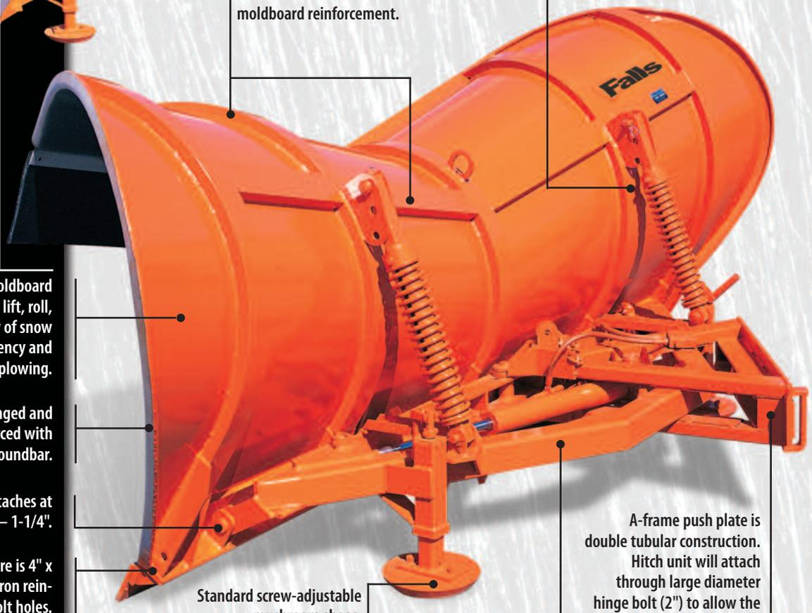
Precise moldboard curvature provides lift, roll, and throw of snow for maximum efficiency and easier plowing.
