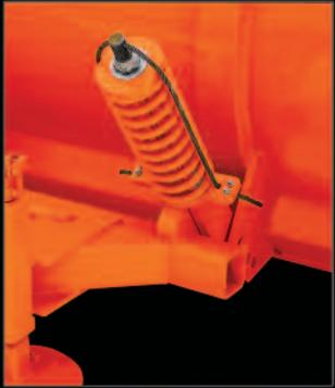
Optional slotted trip (shown) or compression spring trip tilting bars.
