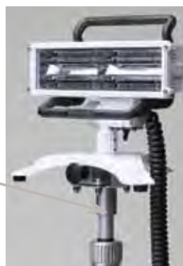
Finished assembly of ground tripod mounted on top of folding tripod pole with ground tripod mount.
