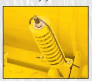
Optional slotted trip (shown) or compression spring trip tilting bars.
