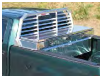
Extra Deep Crossbody Toolbox with a single diamond plate Aluminum Lid
