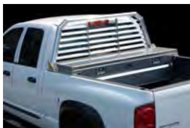
Low-Pro Crossbody Toolbox with a single diamond plate Aluminum Lid
