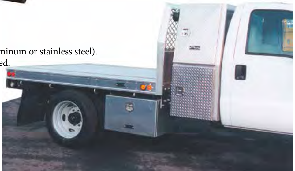
15 x 15 Aluminum or Steel Underbody Box* with single drop down door in aluminum or steel available in 18", 24", 30" lengths
